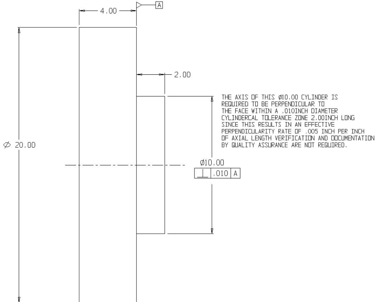
DS-703 EXAMPLE 2 EFFECTIVE RATE CONTROL OF PERPENDICULARITY
