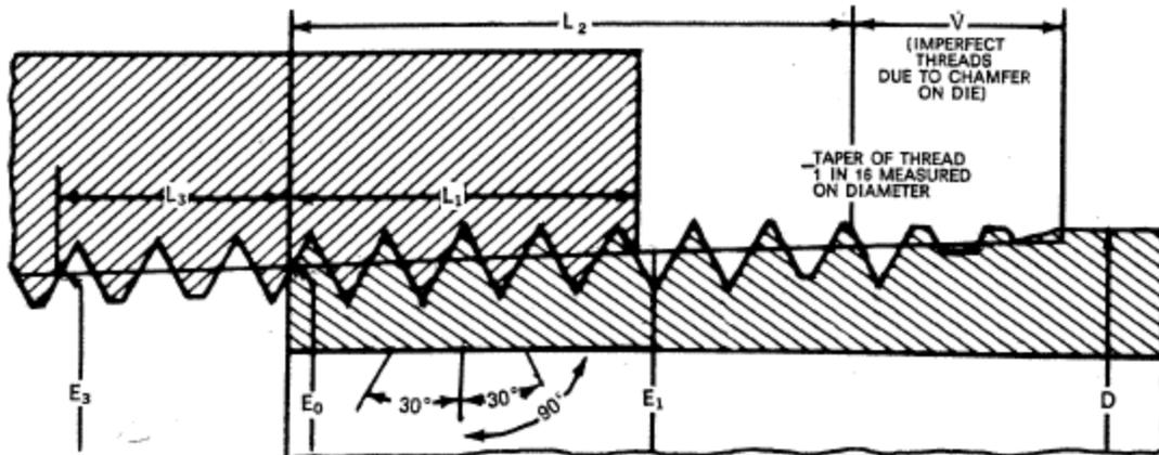
**BASIC DIMENSIONS, ANSI STANDARD TAPER PIPE THREAD<sup>1</sup>**
