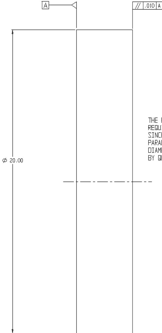
THE FACES OF THIS Ø20.00 CYLINDER ARE REQUIRED TO BE PARALLEL WITHIN .010INCH. SINCE THIS RESULTS IN AN EFFECTIVE PARALLELISM RATE OF .0005 INCH PER INCH OF DIAMETER, VERIFICATION AND DOCUMENTATION BY QUALITY ASSURANCE ARE REQUIRED.
